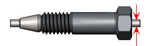
**CRIMP HERE WITH PLIERS** TO SLIGHTLY DEFORM THE **PLUG END AND HOLD** THE PARTS TOGETHER
